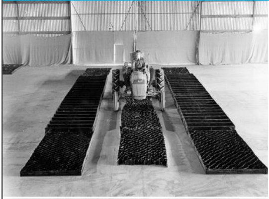
Fertiliser spreader testing in the still air lab
